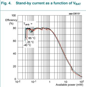
Fig. 6. Efficiency as a function of available power
