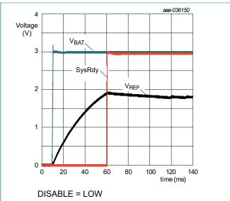
Fig. 5. Start-up sequence; V<sub>REF</sub>, V<sub>BAT</sub> and SysRdy as a function of time
