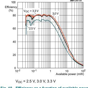
Fig. 10. Efficiency as a function of available power
