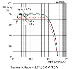
Efficiency as a function of input current
