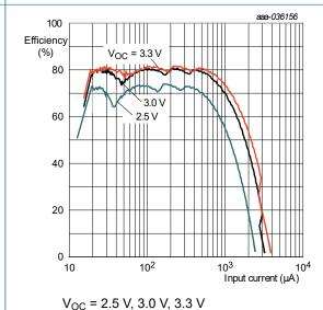
Fig. 11. Efficiency as a function of input current
