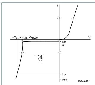
Fig. 3. V-I characteristics for a unidirectional ESD protection diode
