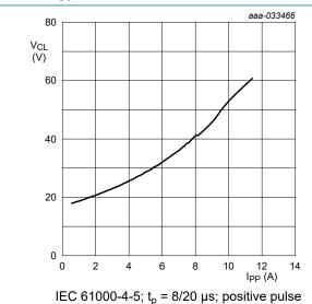
Fig. 6. Dynamic resistance with positive clamping; typical values
