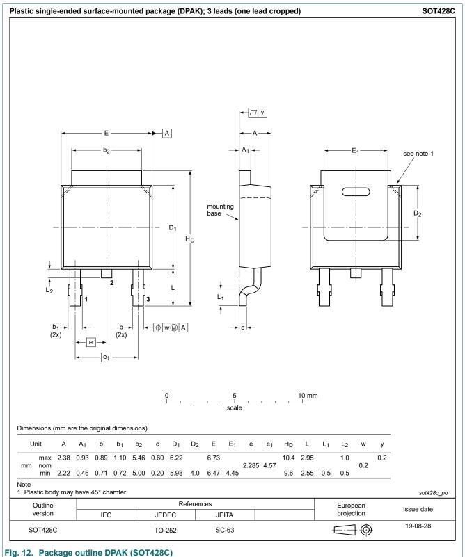
80 V, 8 A PNP high power bipolar transistor
