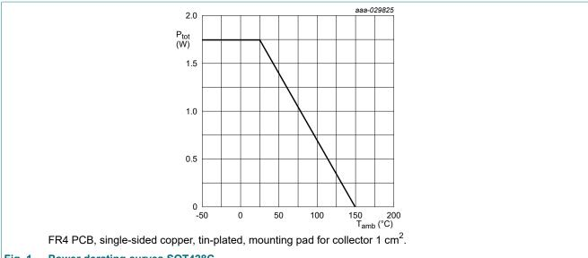
Fig. 1. Power derating curves SOT428C
