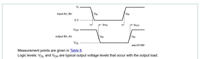
Fig. 5. The data input (An, Bn) to output (Bn, An) propagation delay times
