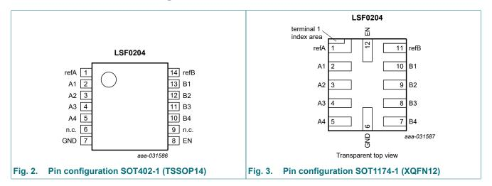
4-bit bidirectional multi-voltage level translator; open-drain; push-pull
