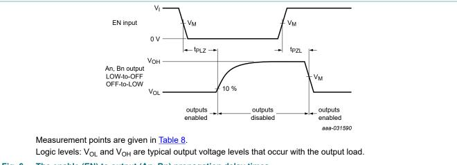
Fig. 6. The enable (EN) to output (An, Bn) propagation delay times
