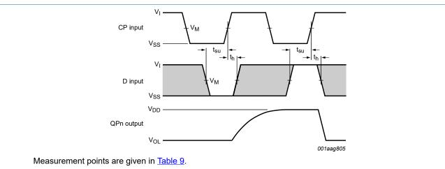
V<sub>OL</sub> is a typical output voltage level that occurs with the output load.
