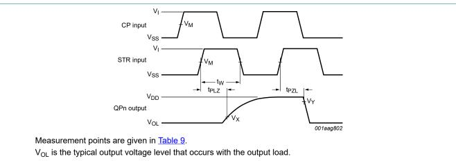
Strobe (STR) to output (QPn) propagation delays and the strobe pulse width Fig. 7.
