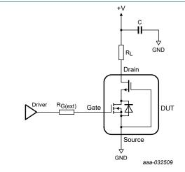
Fig. 16. Switching time test circuit
