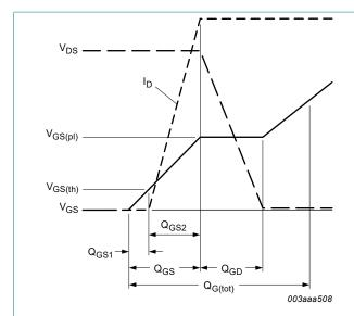
Fig. 13. Gate charge waveform definitions
