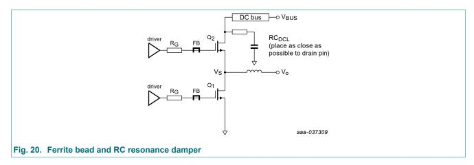
A DC-link resonance damper is recommended in all cases. Optimal is 20 nF in series with 4  $\Omega$ , most easily achieved with parallel combination 10 nF and 8  $\Omega$ . This resonance damper lowers the Q factor of any resonance in the bus. That resonance will act as a load on the high gain amplifier that is the GaN FET and can lead to instability.
