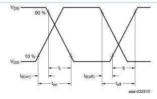
Fig. 17. Switching time waveform
