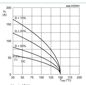
$V_{GS} \ge 10 \text{ V}$  (1) 53.5A DC continuous current has been successfully demonstrated during application tests. Practically the current will be limited by PCB, thermal design and operating temperature.
