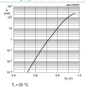
Forward current as a function of forward Fig. 4. voltage; typical values (BZX884S-B/C75)
