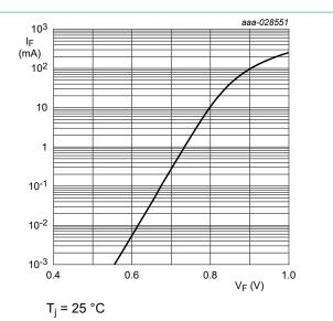
Forward current as a function of forward Fig. 2. voltage; typical values (BZX884S-B/C6V8)
