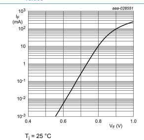
Fig. 3. Forward current as a function of forward voltage; typical values (BZX84-A/B/C6V8)
