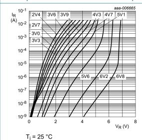
Fig. 8. Reverse current as a function of reverse voltage; typical values (BZX84-A/B/C2V4 to BZX84-A/B/C6V8)
