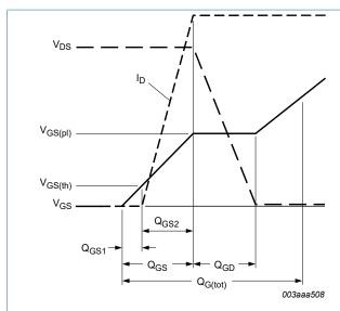
Fig. 14. Gate charge waveform definitions
