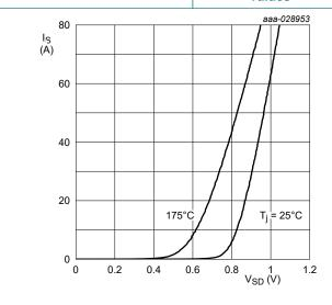
Fig. 16. Source-drain (diode forward) current as a function of source-drain (diode forward) voltage; typical values
