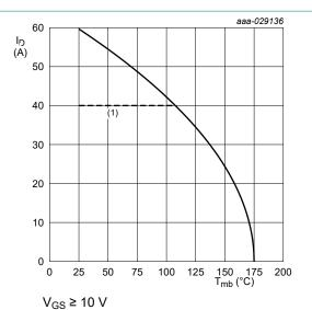
(1) 40A continuous current has been successfully demonstrated during application tests. Practically the current will be limited by PCB, thermal design and operating temperature.
