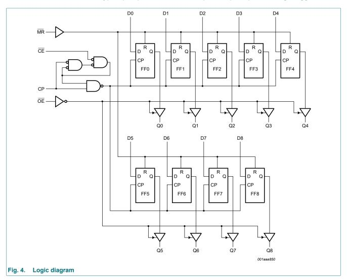
9-bit D-type flip-flop with 5 V tolerant inputs/outputs; positive edge-trigger; 3-state
