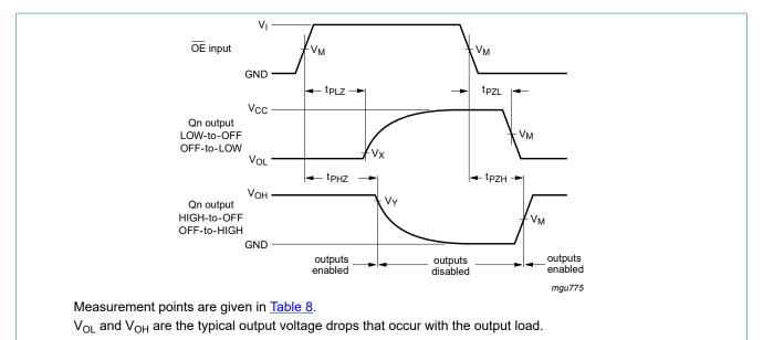
Fig. 10. 3-state outputs enable and disable times
