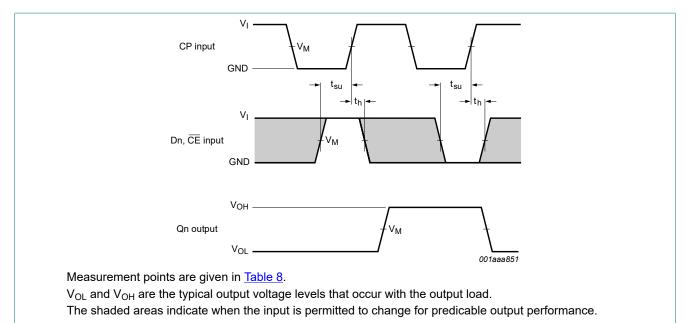
Data set-up and hold times for data and clock enable inputs to clock input Fig. 8.
