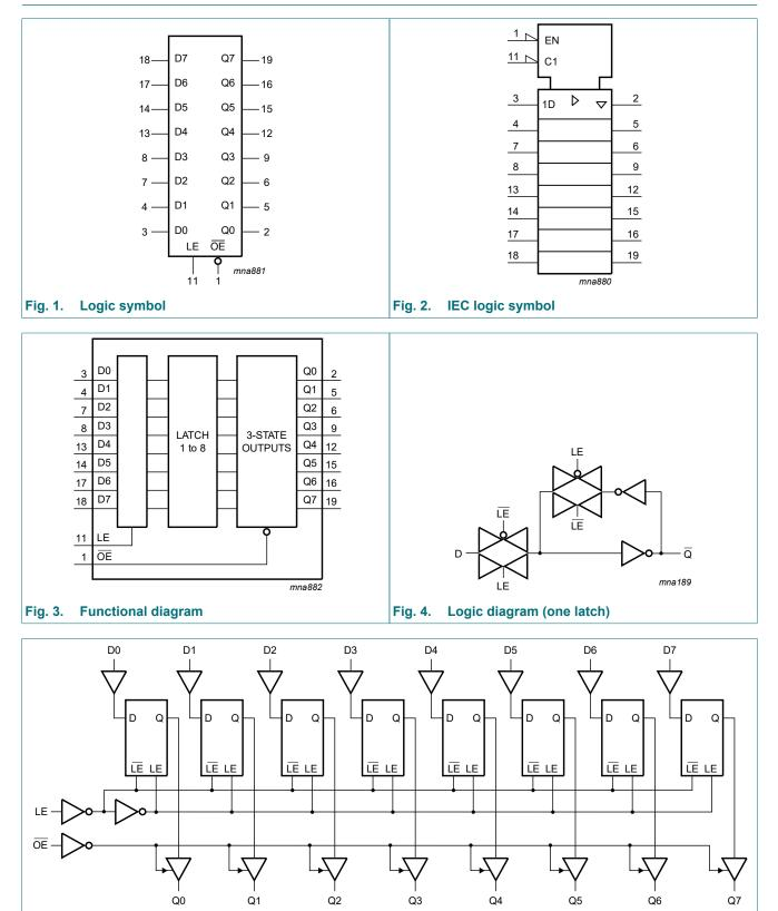
Fig. 5. Logic diagram
