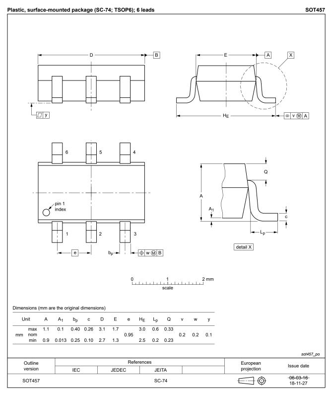
Fig. 7. Package outline SOT457 (SC-74; TSOP6)
