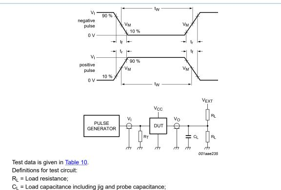
$R_{T}$  = Termination resistance should be equal to output impedance  $Z_{o}$  of the pulse generator;
