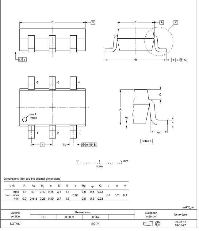
Fig. 11. Package outline SOT457 (SC-74; TSOP6)
