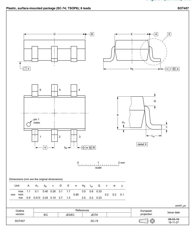
Fig. 9. Package outline SOT457 (SC-74; TSOP6)
