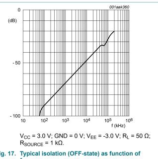
Fig. 17. Typical isolation (OFF-state) as function of frequency
