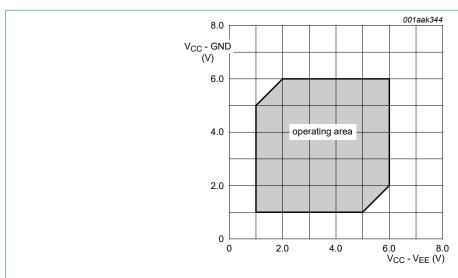
Fig. 5. Guaranteed operating area as a function of the supply voltages
