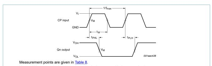
$V_{\text{OL}}$  and  $V_{\text{OH}}$  are typical output voltage levels that occur with the output load.
