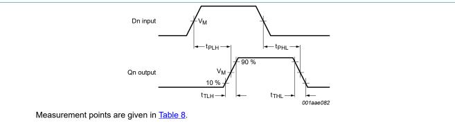
Fig. 7. Propagation delay data input (Dn) to output (Qn) and output transition time
