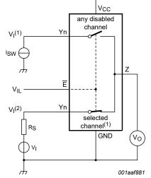
(1) Channel is selected by S0, S1 and S2.  $V_I(1)$  < GND or  $V_I(1)$  >  $V_{CC}$ . GND <  $V_I(2)$  <  $V_{CC}$ .
