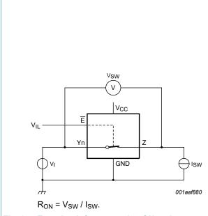
Fig. 6. Test circuit for measuring ON resistance
