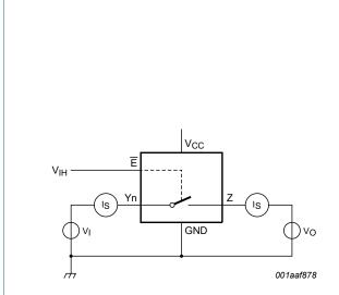
Fig. 4. Test circuit for measuring OFF-state leakage current
