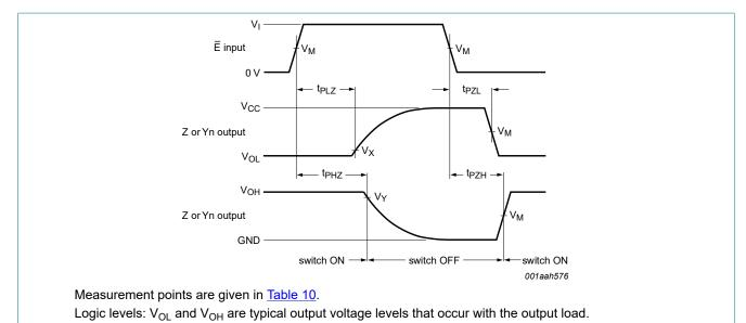
Fig. 10. Enable and disable times
