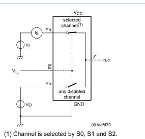
Fig. 5. Test circuit for measuring ON-state leakage current
