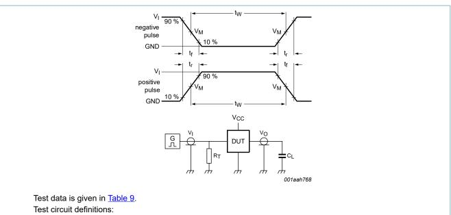
$R_T$  = Termination resistance should be equal to output impedance  $Z_o$  of the pulse generator;
