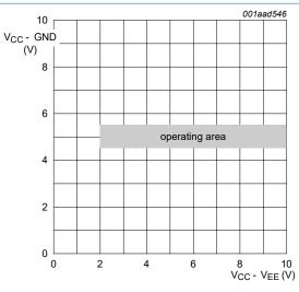
Fig. 6. Guaranteed operating area as a function of the supply voltages for 74HCT4351
