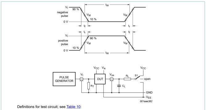
$R_T$  = Termination resistance should be equal to the output impedance  $Z_0$  of the pulse generator;
