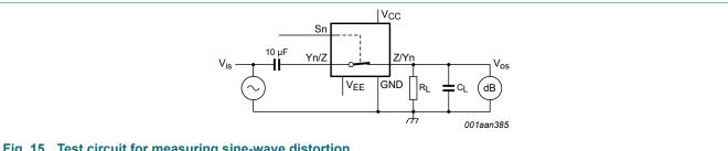
Fig. 15. Test circuit for measuring sine-wave distortion
