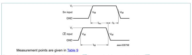
Fig. 13. Set-up and hold times from Sn inputs to  $\overline{\text{LE}}$  input, and minimum pulse width of  $\overline{\text{LE}}$ .
