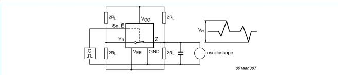
Fig. 17. Test circuit for measuring crosstalk between control input and any switch
