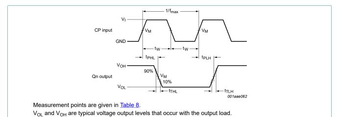
Fig. 7. Propagation delay clock input (CP) to output (Qn), clock (CP) pulse width, output transition time and the maximum clock pulse frequency
