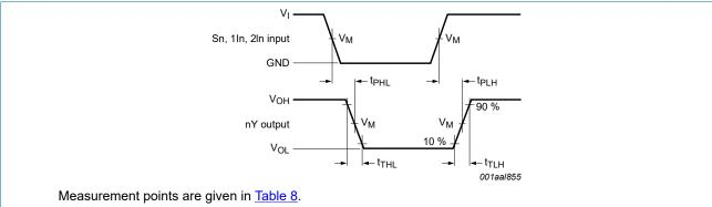
$V_{OL}$  and  $V_{OH}$  are typical voltage output levels that occur with the output load.
