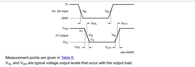
Waveforms showing the input (1In, 2In) to output (1Y, 2Y) propagation delays and output transition times Fig. 6.
