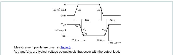
Fig. 7. Waveforms showing the input (Sn, nE) to output (nY) propagation delays
