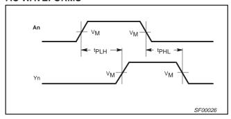
Waveform 1. Propagation delay for non-inverting outputs NOTE:
