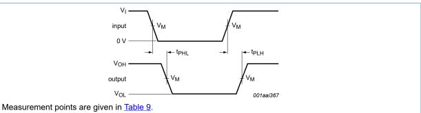
Logic levels:  $V_{OL}$  and  $V_{OH}$  are typical output voltage levels that occur with the output load.
