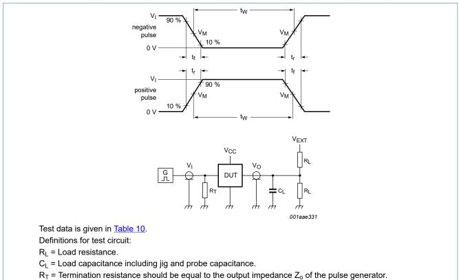
V<sub>EXT</sub> = External voltage for measuring switching times.
