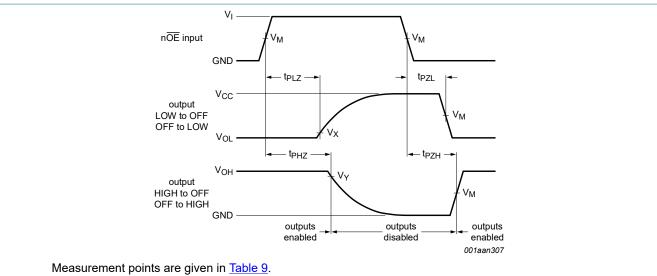
Logic levels: V<sub>OL</sub> and V<sub>OH</sub> are typical output voltage levels that occur with the output load.
