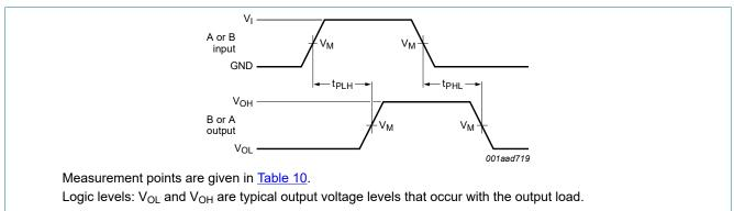
Fig. 11. The data input (A or B) to output (B or A) propagation delays
