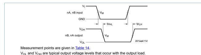
Fig. 6. The data input (nA, nB) to output (nB, nA) propagation delay times
