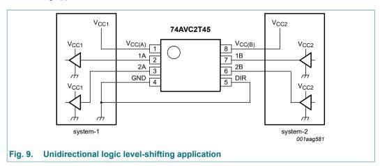
Table 16. Unidirectional logic level-shifting application
