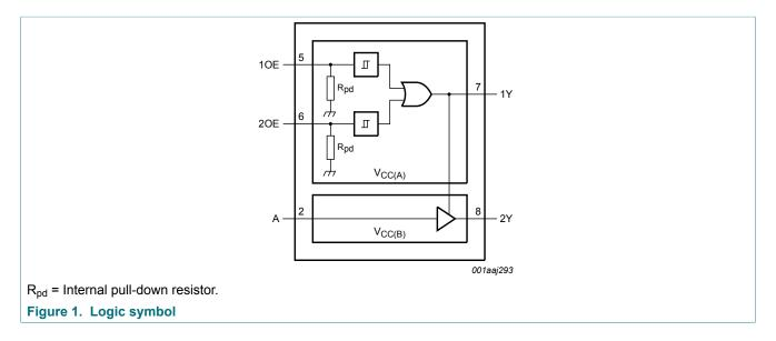
Low-power dual supply buffer/line driver; 3-state
