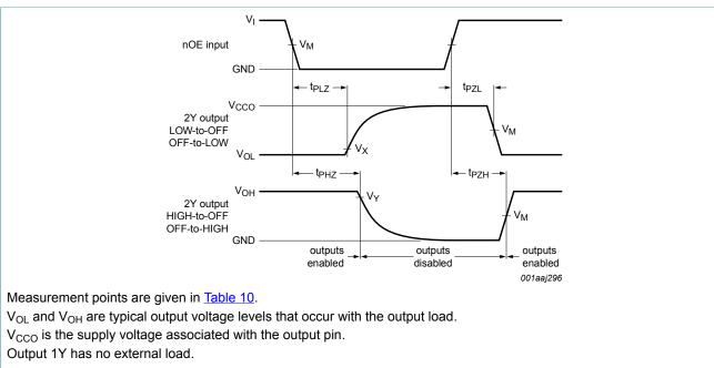
Figure 8. Enable and disable times
