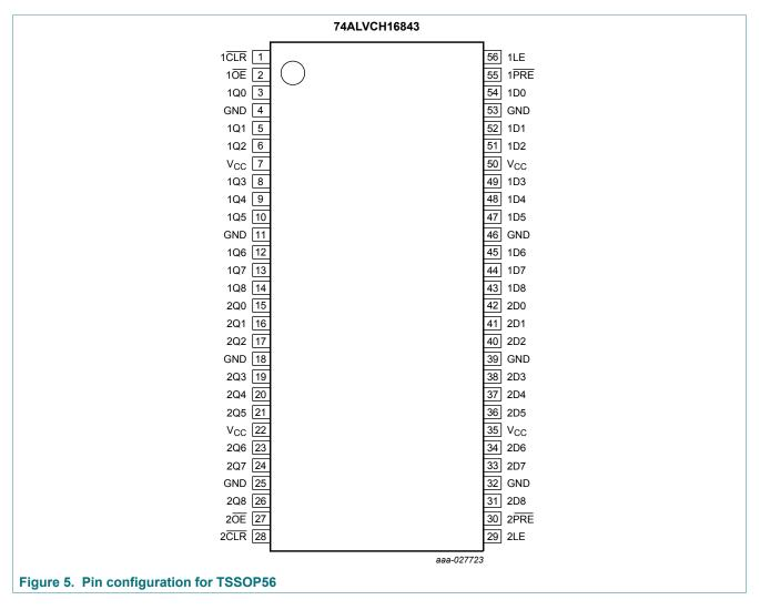
18-bit bus-interface D-type latch; 3-State
