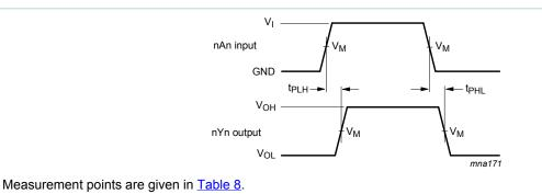
$V_{\text{OL}}$  and  $V_{\text{OH}}$  are typical voltage output levels that occur with the output load.
