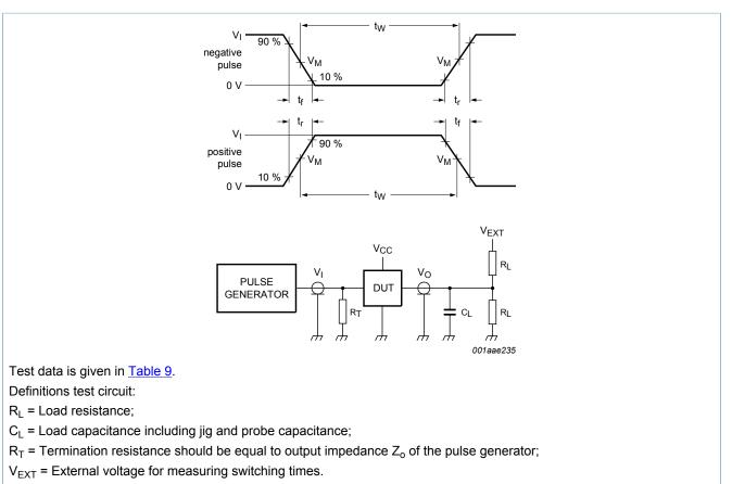
Figure 10. Test circuit for measuring switching times
