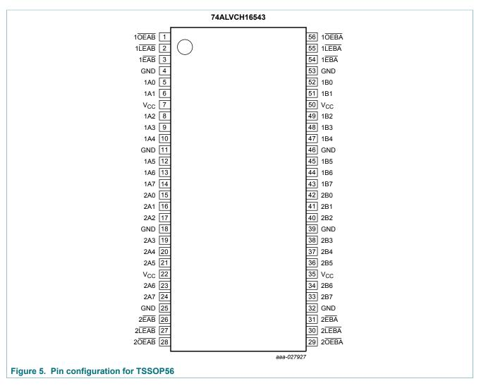
16-bit D-type registered transceiver; 3-state
