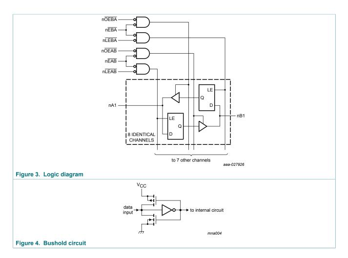
16-bit D-type registered transceiver; 3-state
