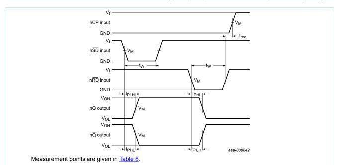
Fig. 6. Set  $(n\overline{SD})$  and reset  $(n\overline{RD})$  input to output  $(nQ, n\overline{Q})$  propagation delays, set  $(n\overline{SD})$  and reset  $(n\overline{RD})$  pulse widths and  $n\overline{RD}$  to nCP recovery time
