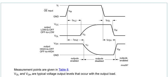
Fig. 4. Enable and disable times
