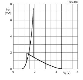
Typical 74AHCT1G17 transfer characteristics;  $V_{CC} = 4.5 \text{ V}$
