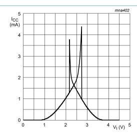
Fig. 7. Typical 74AHC1G17 transfer characteristics;  $V_{CC}$  = 4.5 V
