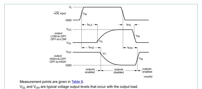
Fig. 5. Enable and disable times
