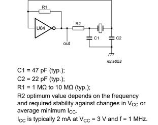
Fig. 12. Crystal oscillator configuration
