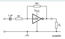
Maximum  $V_{o(p-p)} = V_{CC}$  - 1.5 V centered at 0.5 ×  $V_{CC}$ .
