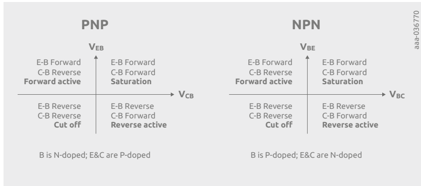
Figure 18 | Voltage values determining the four different regions of operation
