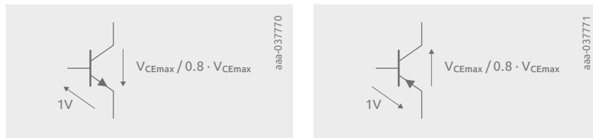
Figure 7 | Bis setting during HTRB/H3TRB
