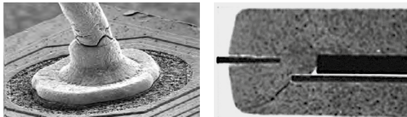
Figure 2 | Potential failure modes can be caused by manufacturing: broken stitch (left), package crack (right)
