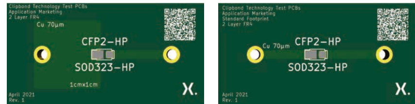
Figure 51 | Example CFP2-HP test boards: 1cm 2 mounting pad for cathode vs. standard footprint.
