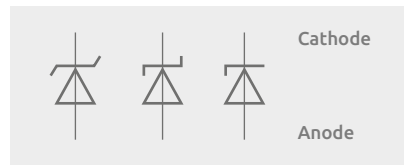
Figure 39 | Common symbols for a Zener diode.
