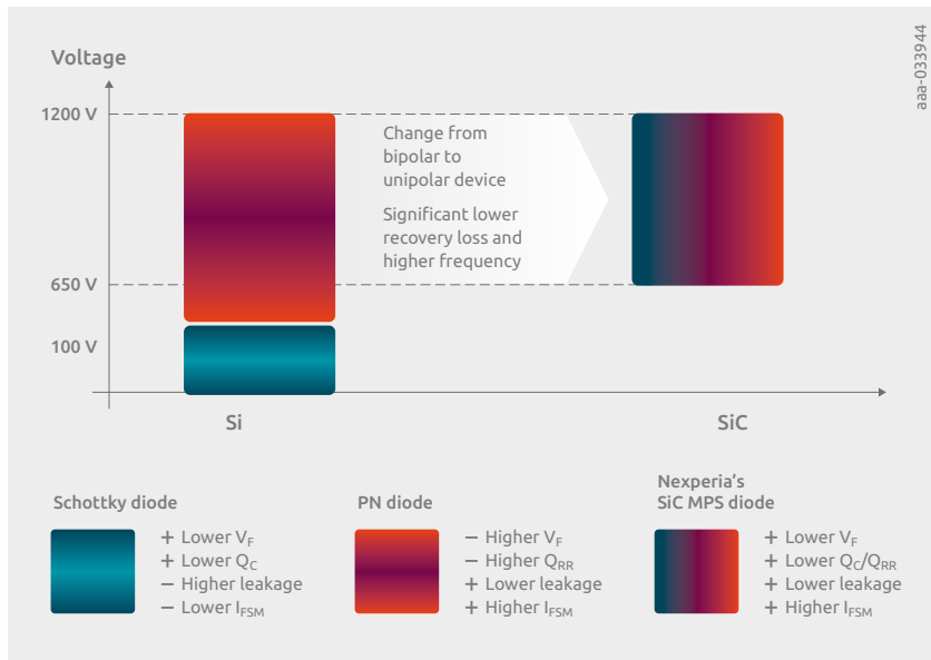
Figure 28 | SiC MPS diode.
