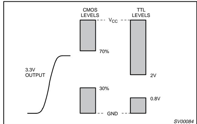
Figure 1. Switching Levels
