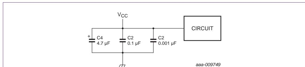
**Fig 3. Multiple capacitors used to bypass different frequencies**
