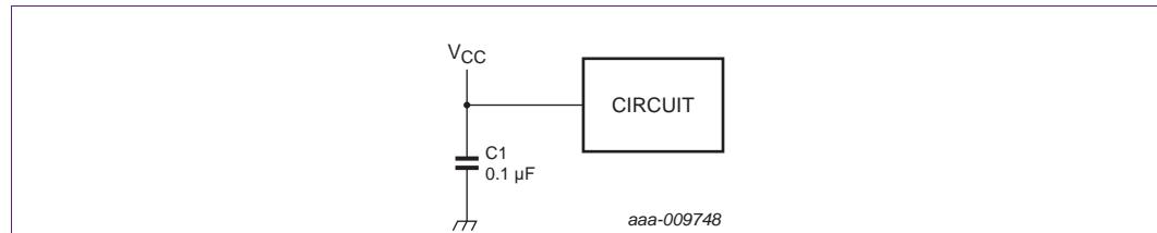
**Fig 2. Single bypass capacitor for low current and high frequency noise applications**
