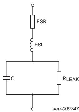
**Fig 1. Equivalent circuit of a capacitor**
