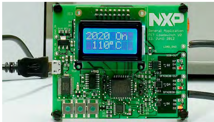
Fig 11. Test with DFN3333-8 (SOT873-1) package
