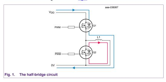
In this application note, Q1 and Q2 are BUK7Y2R0-40H devices. Other devices could be considered. Inductor L1 could be connected to  $V_{DD}$  rather than 0 V.
