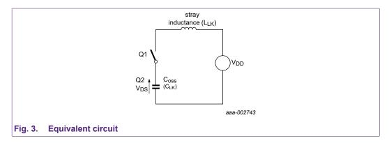
We are primarily interested in the parasitic elements in the circuit:
