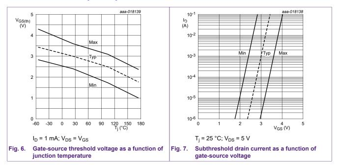
Fig. 6 shows the variation in the threshold voltage for the typical and limit devices over the rated temperature range. All the MOSFETs are guaranteed to have a threshold voltage between the lines.
