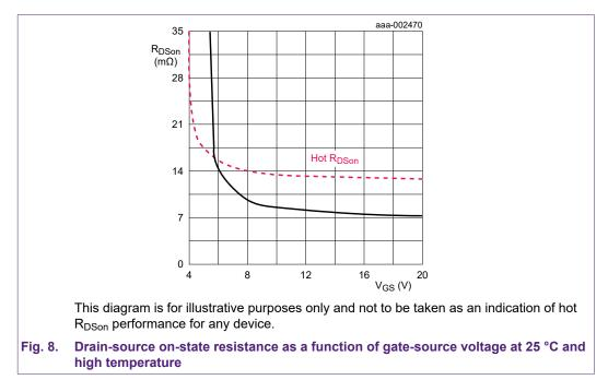
If an application requires good  $R_{DSon}$  performance for lower gate-source voltages, then MOSFETs are made with lower threshold voltages, e.g. the BUK9Y12-55B (logic level MOSFET). However, the lower threshold voltage of such a device means that it has a lower headroom for its off-state at high temperature. This lower headroom often means that a device with a higher threshold voltage is needed.
