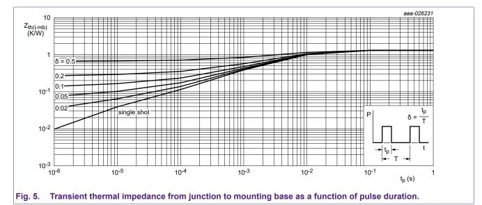
Thermal resistance ( $R_{th}$ ) and thermal impedance ( $Z_{th}$ ) are related because the thermal resistance is the steady-state measure of how the device blocks heat flow. Thermal impedance is how the device responds to transient thermal events. It involves different thermal capacities of parts of the device and the thermal resistances between these parts. Under DC conditions,  $Z_{th}$  is equal to  $R_{th}$ . Equation (4) represents the temperature rise for a particular power dissipation:
