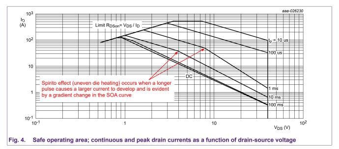
The SOA curves show the voltage allowed, the current and time envelope of operation for the MOSFET. These values are for an initial  $T_{mb}$  of 25 °C and a single current pulse. This is a complex subject which is further discussed in the appendix (Section 3.1).
