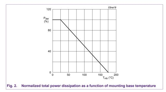
The curves provided in Fig. 1 and Fig. 2 are read in conjunction with the limiting values tables. The information extracted, assists in calculating the maximum current allowed and the power dissipation with respect to temperature.
