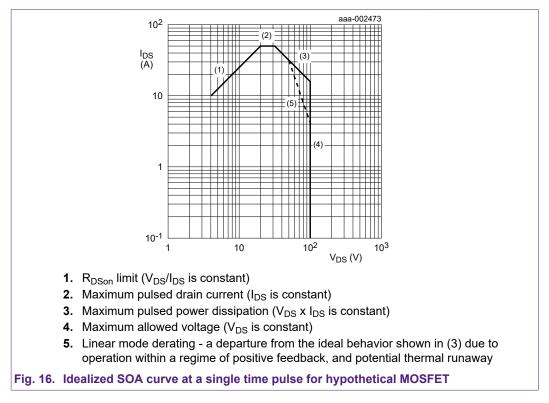
The dashed line (5) is to emphasize where the curve deviates from the ideal. In reality, there is a single curve with a change of gradient where the linear mode derating becomes important.
