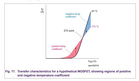
The resistance increase dominates at high currents, meaning that localized heating leads to lower currents. The threshold-voltage drop dominates at low currents, meaning that localized heating lowers the threshold voltage. This condition effectively turns on the device more, leading to higher currents and a risk of thermal runaway.
