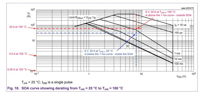
The  $I_D$  derating of the SOA curve at 100 °C is shown in Fig. 18.
