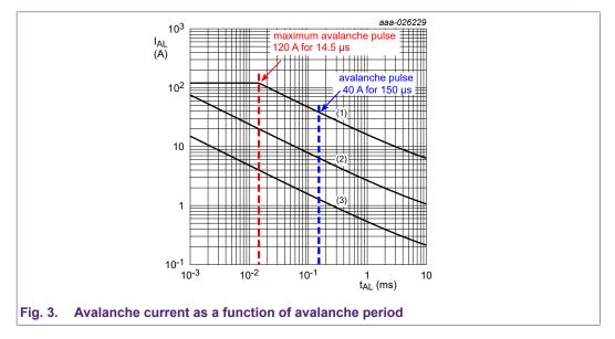
A simple example for the BUK7Y3R5-40H, using the information in *AN10273*, is extracted from the limiting values <u>Table 3</u>:
