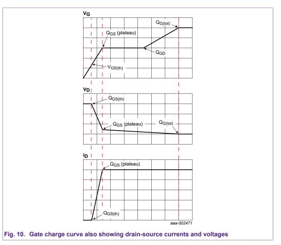
Due to capacitance variation with voltage and current, it is better to look at the gate charge data rather than the capacitance data when determining switching performance. This is especially true if the gate-driver circuit for the MOSFET is limited to a particular current, and a rapid switch is required.
