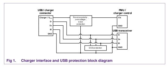
As shown in <u>Figure 1</u> a complete protection solution for the USB and charger port consists of two blocks. The first block protects the USB  $V_{BUS}$  or charger interface against reverse polarity and overvoltage. The second block protects the USB data lines and the downstream components against damage from ESD. The subsequent sections illustrate the protection concepts of these blocks in more detail.
