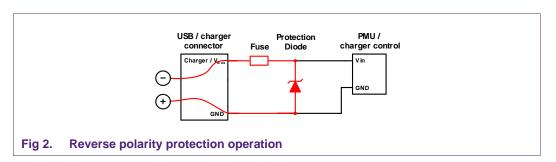
The positive voltage supplied to the GND input of the charger can pass through the forward biased protection diode and the protective fuse, back to the charger negative pole. In this concept the protection diode needs to be able to conduct high currents only until the fuse clears. Fast reacting fuses can clear in 100 ms. Section 3.4 describes protection diodes that are able to conduct up to 5 A for the necessary period of time.
