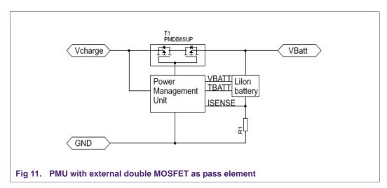
By connecting the MOSFET in this configuration, the Schottky diode has been eliminated. If both gates can be controlled independently, the PMU can control the charging current and also the discharging current if the USB port has to supply power. It is a superior solution compared to using a MOSFET-Schottky diode module, but it does cost more.
