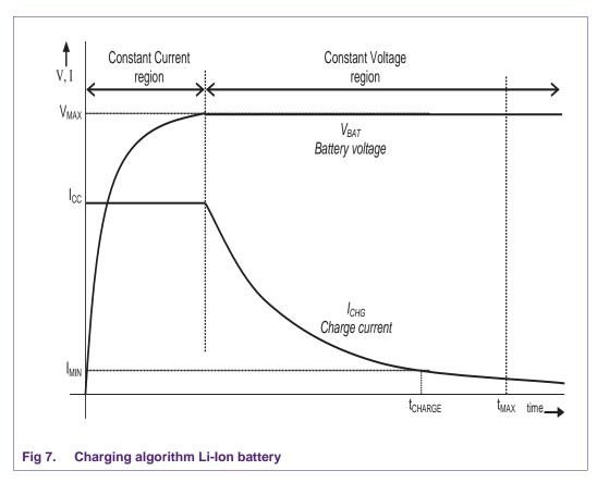
The value of  $V_{MAX}$  and  $I_{CC}$  depends on the type of battery that is used. The maximum charge rate in CC mode is 1C, where 1C indicates the capacity of the battery e.g. 1000 mAh. The value of  $V_{MAX}$  is typically in the range of 4.1 to 4.2 volts.
