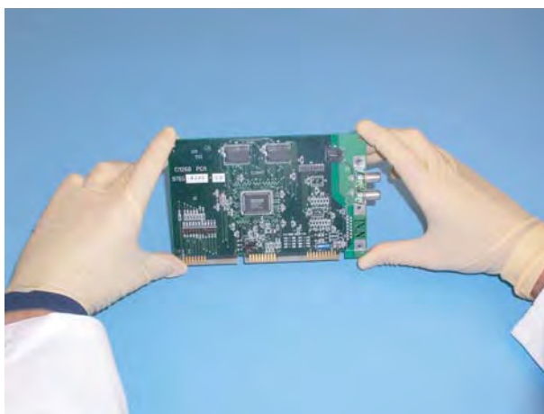
Fig 29. Manual handling of an assembled board
