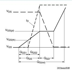
Fig 14. Gate charge waveform definitions
