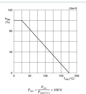
Normalized total power dissipation as a Fig 2. function of mounting base temperature
