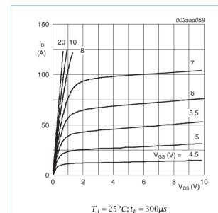
Output characteristics: drain current as a Fig 5. function of drain-source voltage; typical values
