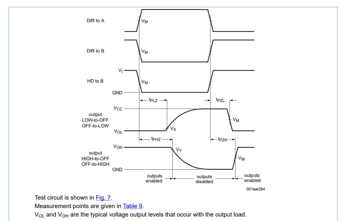
Fig. 6. Enable and disable times
