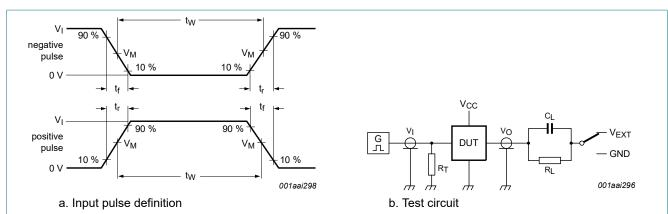
$C_L$  = load capacitance includes jig and probe capacitance.
