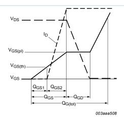
Fig. 13. Gate charge waveform definitions
